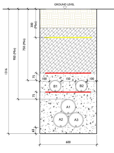
A = 160mm: Outer Diameter HDPE ESB Approved Duct, SDR=21
